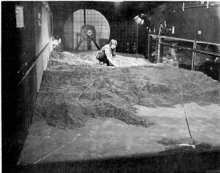
Figure 3.2-2 Photograph of Terrain Model in the Environmental Wind Tunnel
